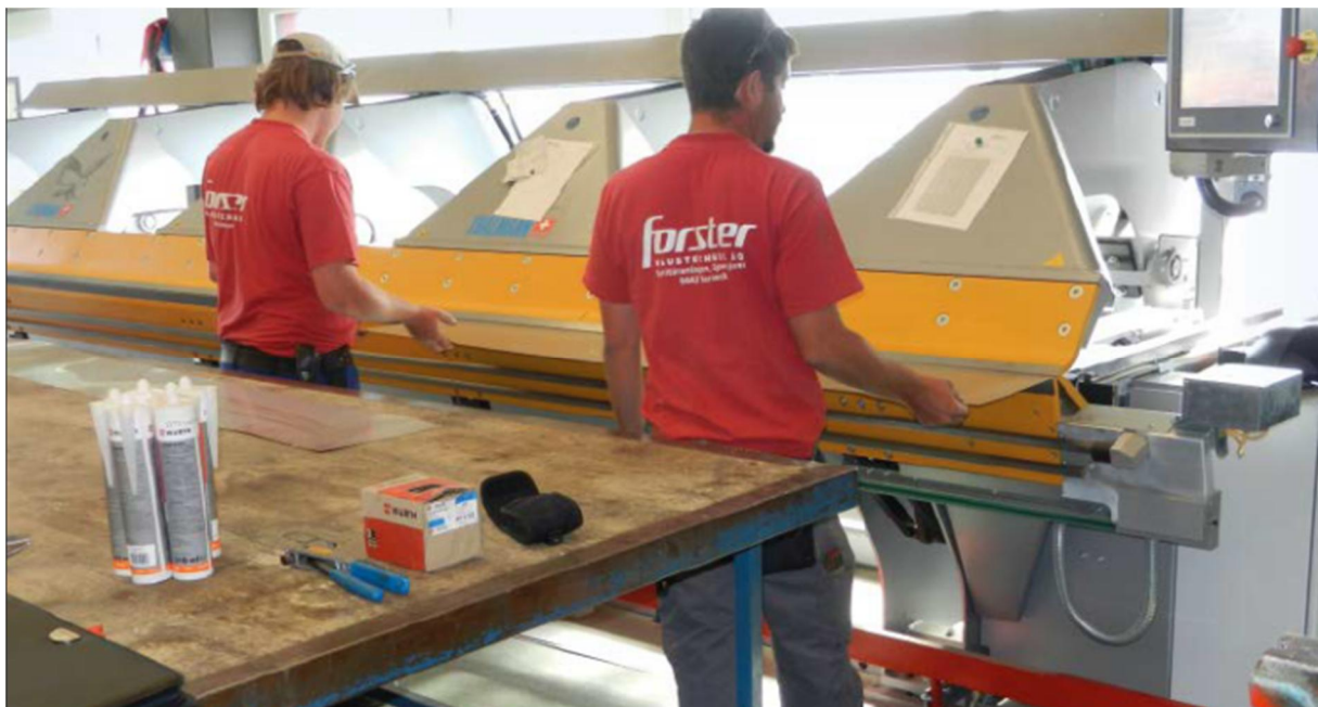
Forster Haustechnik AG uses a modern swing-folding machine to create façades. (image: Carl Geisser AG)
