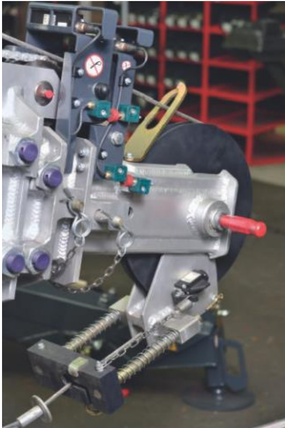
Wireless magnetic switches monitor the extension status of individual telescopic parts
