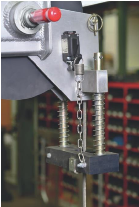
A wireless pull wire switch causes the winch to stop when the hook block reaches its upper limit
