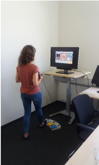
Prototype for different ways of controlling equipment during spinal surgery. Here foot control is being used.
