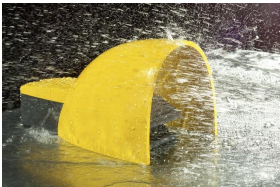
A good idea, but not 100 % meaningful for switchgear in adverse environments: corrosion tests in the laboratory
