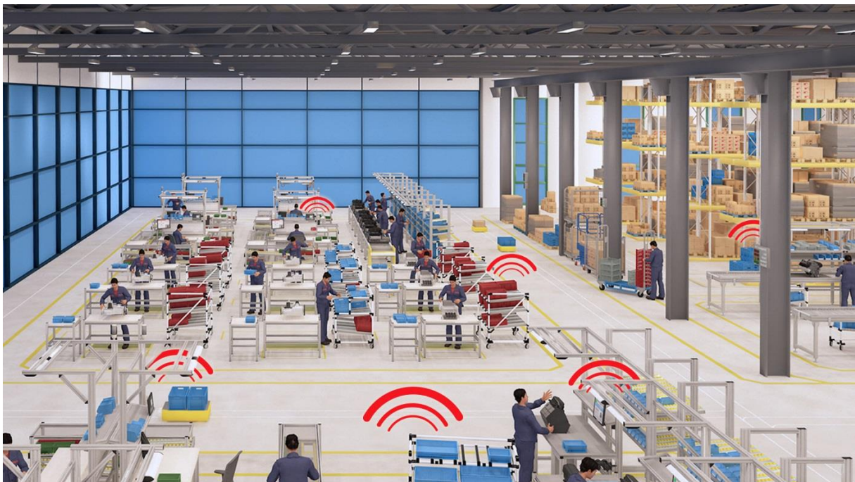
01 The wireless network collects (remote) signals in the field and transmits them via a Sensor Bridge to the IT infrastructure of the user.
