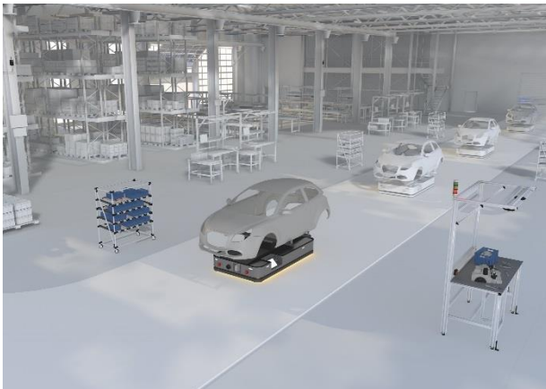
Fig 2 In pilot factories, car manufacturers are testing flexible serial production without stationary conveyors, using automated guided vehicles.
