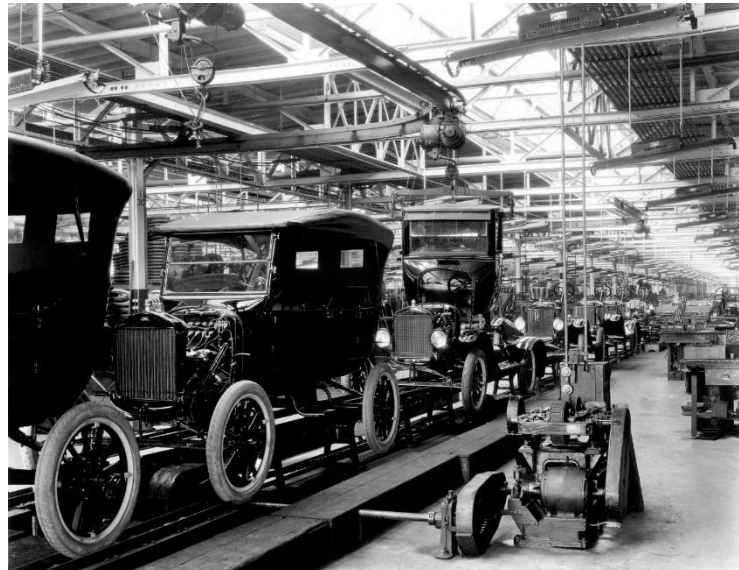
Fig 1 Ford introduced mass production with fixed conveyors back in 1918. Many state-of-the-art automotive manufacturers are currently installing more flexible AGV in their assembly processes.
