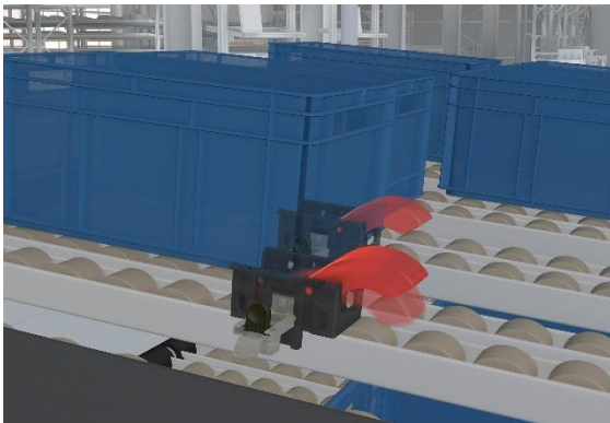
05 Wireless sensors developed specifically for eKanban systems detect the occupancy of rack slots and notify the warehouse management system via the wireless infrastructure
