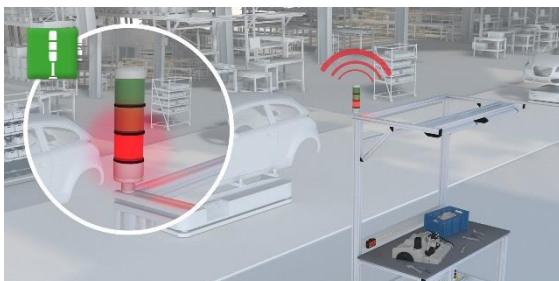
The wireless system can also assume additional tasks, e.g. the integration of Andon systems
