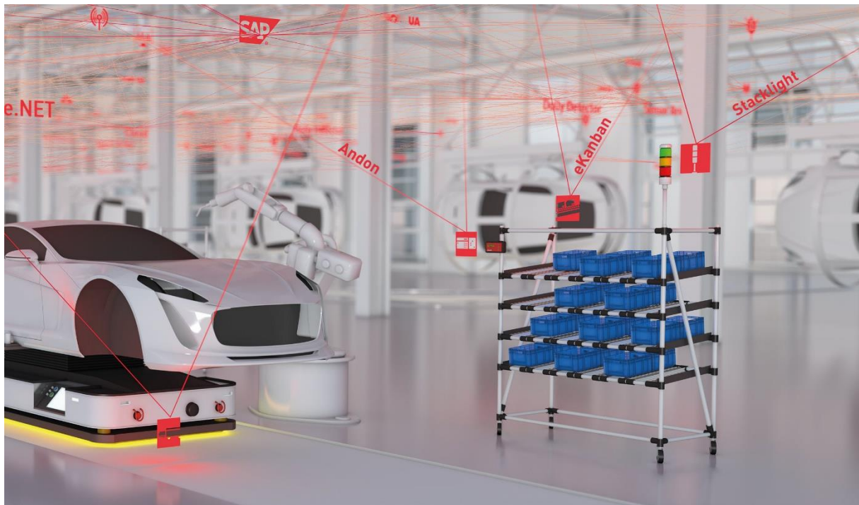
The wireless network can integrate e.g. mobile eKanban racks in the inventory management, leading to a materials requisition system which is flexible and "seamless"
