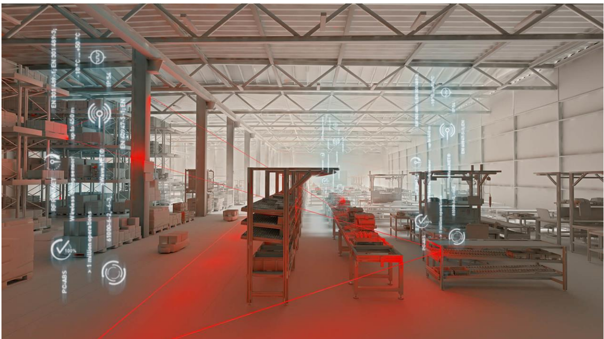
Signals from wireless sensors at the shop floor level are received by Access Points and passed on to a Sensor Bridge.
